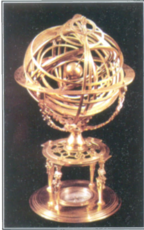
A sixteenth-century Flemish armillary sphere showed a geocentric model with seven nesting planetary rings.
